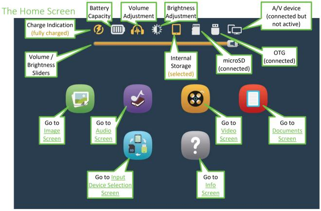
Above: Leaf is connected for charging (completed), an external audio device is connected, A/V device is connected (but not active), the volume is being adjusted, external microSD and OTG are connected but Internal Storage is the selected input.
