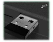
To connect an OTG device, gently insert it into the <u>Type-A connector</u> next to the microSD card reader slot. It will only fit in correctly when the side with the 2 openings is facing you (per the illustration).
