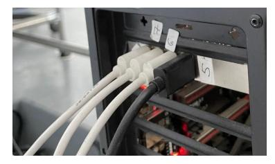
One of the SGS computers is configured to use 96 mapped folders (6 hubs with 16 ports each). Each hub is connected to a USB port managed by a separate USB controller internally. The 6 USB ports in use are (2) from the motherboard and (4) from the PCI Express card shown above.
