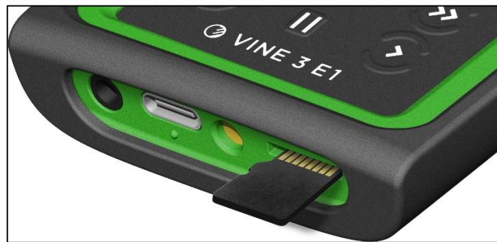
To remove the *microSD* card, gently push it in. The reader will unlock and push the card out so you can remove it. *Take care that the card doesn't suddenly spring out!*
